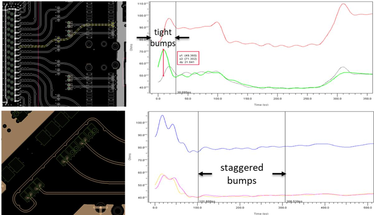
Figure 13: Correct (lower) and incorrect (upper) p/n length matching
