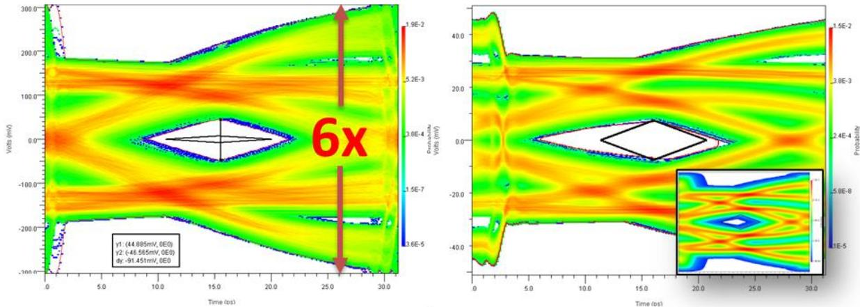
Figure 21: Eye diagrams, Xconn IC (left) and Reference (right) EQ
