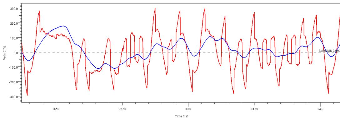
*Figure 8: Rx equalization recovering a valid signal (red) from its input (blue)*
