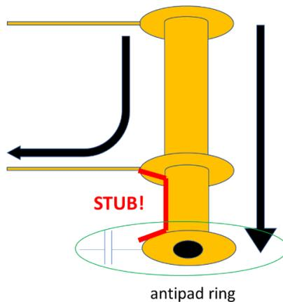
Figure 14: Stub lengths include pads, if not removed
