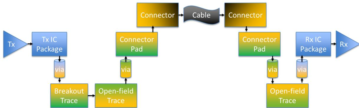
Figure 10: Typical set of discontinuities in a Gen5 Tx to Rx path
