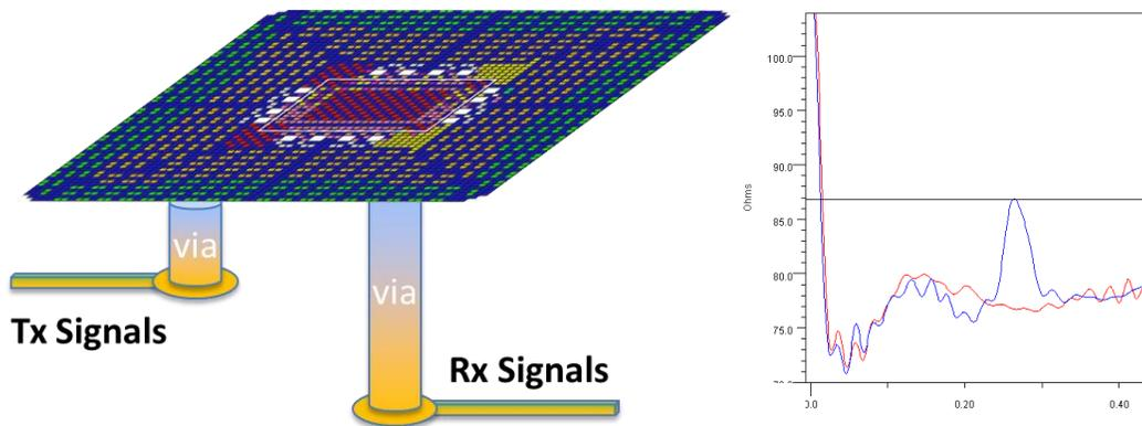
Figure 11: ViP orientation (left) and impedance (right)
