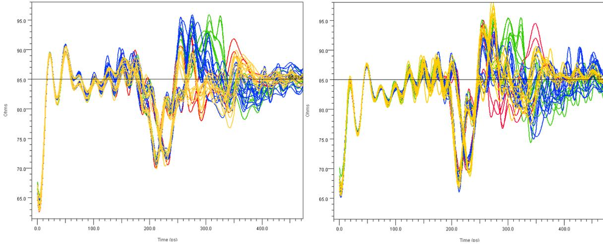
*Figure 15: Cable connector impedance measurements, four vendors (by color)*
