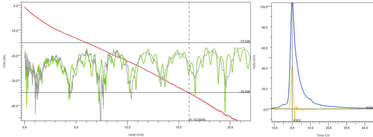
*Figure 19: Maximum IL Path Characteristics*
